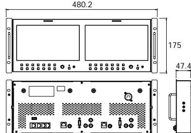
A brand-new rack-mount monitor with 2 × 9" LCD screens, which has the same high performance display as LVM-095W-N with full HD resolution and wide viewing angle capability. It supports SDI in/out and HDMI input.
