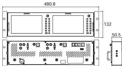
A brand-new rack-mount monitor with 2 × 7" LCD screens, which has the same high performance display as LVM-074W. Wide viewing angle IPS LCD with 1024 x 600 resolution. It supports SDI in/out and HDMI input.
